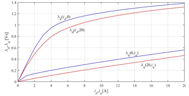
Fig. 2. 3-kW SynRM current-to-flux-linkage map evaluated from experiments.
