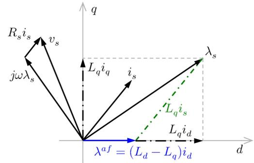
Fig. 5. Active flux definition in the  $dq$  axes frame.
