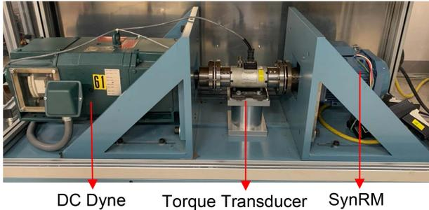
Fig. 13. Experimental dyne setup.
