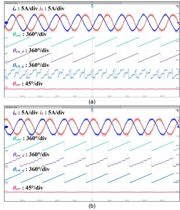
**Fig. 16.** Back EMF-based angle detection at no-load condition. (a) Active  $d$  flux. (b) Active  $q$  flux. Horizontal axis scale: **40 ms/div**.
