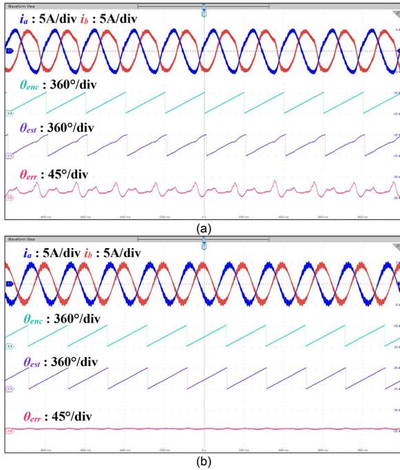
**Fig. 15.** HFI angle detection with 25% rated load. (a)  $i_d = 4$  A and  $i_q = 2.23$  A. (b)  $i_d = 1.76$  A and  $i_q = 4.0$  A. Horizontal axis scale: **200 ms/div**.
