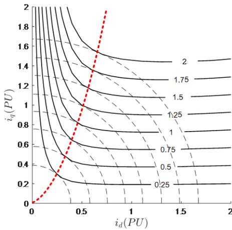
Fig. 4. 3-kW SynRM constant torque curve and MTPA curve. Red dotted line is the MTPA trajectory, solid lines are the torque contours, and dashed lines are the current—magnitude contours.
