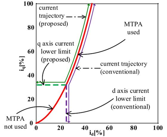
Fig. 11. Proposed minimum  $q$ -axis current trajectory as well as the conventional trajectory defined by a minimum  $d$ -axis current.
