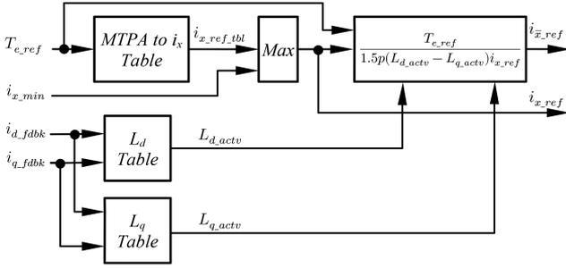
Fig. 12. Current reference generation for a given torque reference. For conventional active  $d$  flux,  $i_x = i_d$  and  $i_{\bar{x}} = i_q$ . For the proposed active  $q$  flux,  $i_x = i_q$  and  $i_{\bar{x}} = i_d$ .
