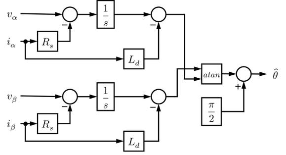
Fig. 10. Rotor position estimation based on the proposed active  $q$  flux.
