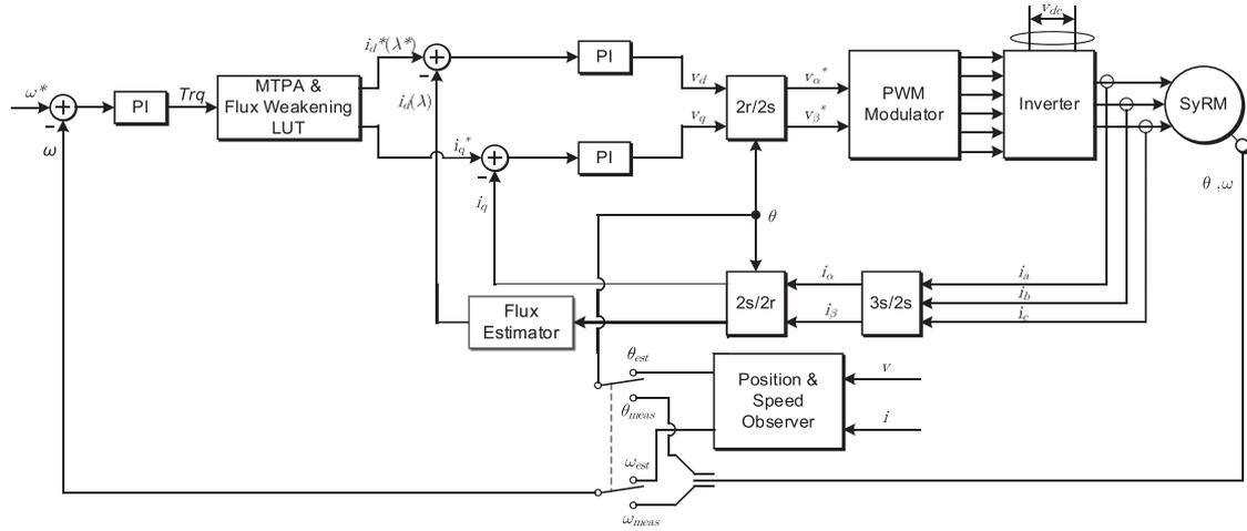
Fig. 3. SynRM FOC control block diagram.
