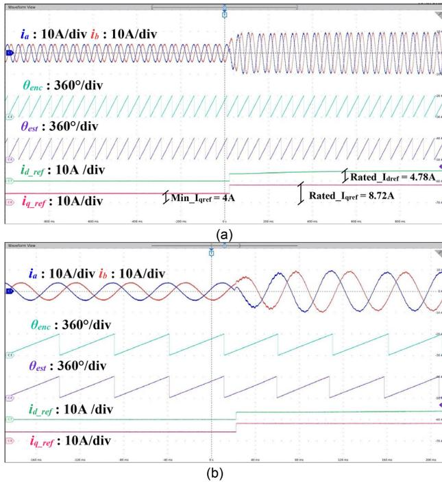
Fig. 19. 0%–100% step load test with the proposed active  $q$  flux concept. (b) is the zoomed view of (a) at the step load moment. (a) (200 ms/div). (b) (40 ms/div).
