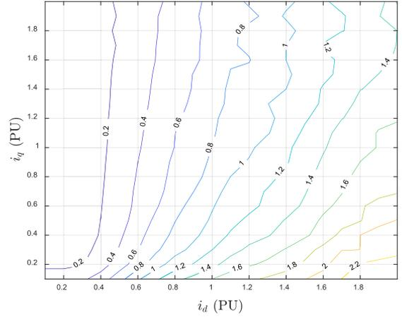
Fig. 7. Saliency ratio on  $i_d$ - $i_q$  current vector plane based on the transient inductance. Note that the saliency ratio contours shown in the figure may deviate away from the actual saliency ratio of the machine when  $|i| \approx 0$  primarily due to testing granularity and measurement.
