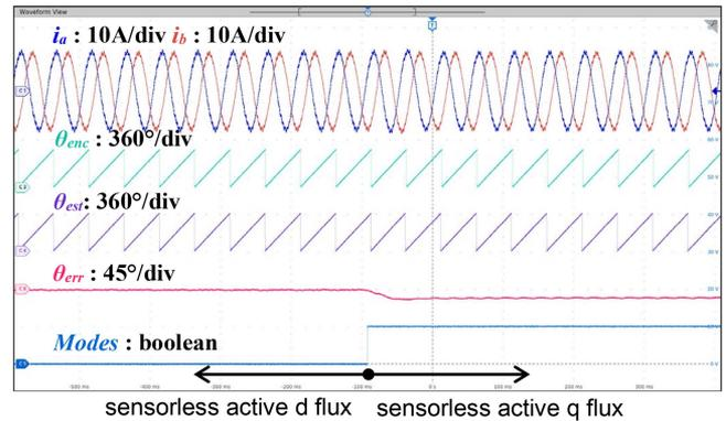
**Fig. 17.** Back EMF-based angle detection with active  $q$  flux concept at rated torque condition. Horizontal axis scale: **100 ms/div**.
