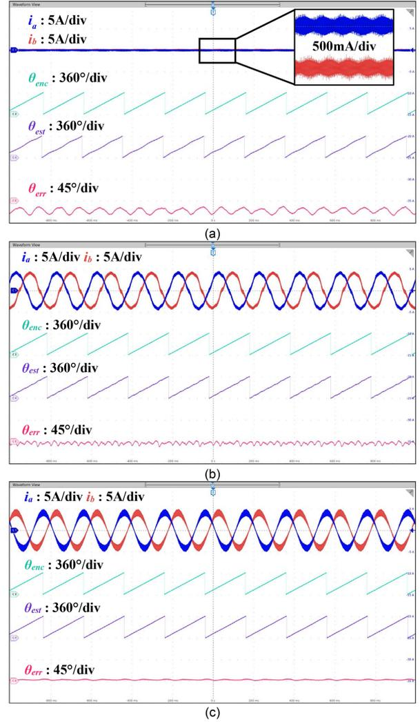
Fig. 14. HFI angle detection with zero torque output. (a). Original with 0  $i_d$  and 0  $i_q$ . (b) Active  $d$  flux with 40%  $i_d$  current and zero  $i_q$  current. (c) Active  $q$  flux with 40%  $i_q$  and zero  $i_d$  current. Horizontal axis scale: 200 ms/div.
