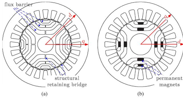
Fig. 1. SynRM and IPM motor stator and rotor cross-sectional lamination [35].
